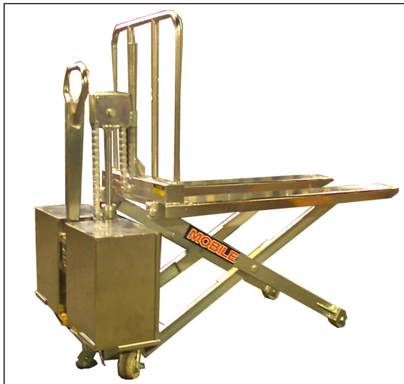
**Brake:** The brake system is designed so the operator can engage the hand lever operated brake at any time - raised or not. The friction brake incorporates a foot pad that is forced to the floor with high pressure from linkage, immobilizing the unit.
