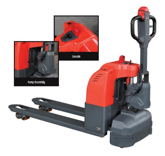
EFET33N is a full electric pallet truck designed as an economic alternative to more expensive fully electric models. These units feature powered operation for lifting and lowering loads, and self-propelled movement for easy transporting of goods. The compact and light design is suitable for a variety of light-duty applications in warehouses or similar environments. The
