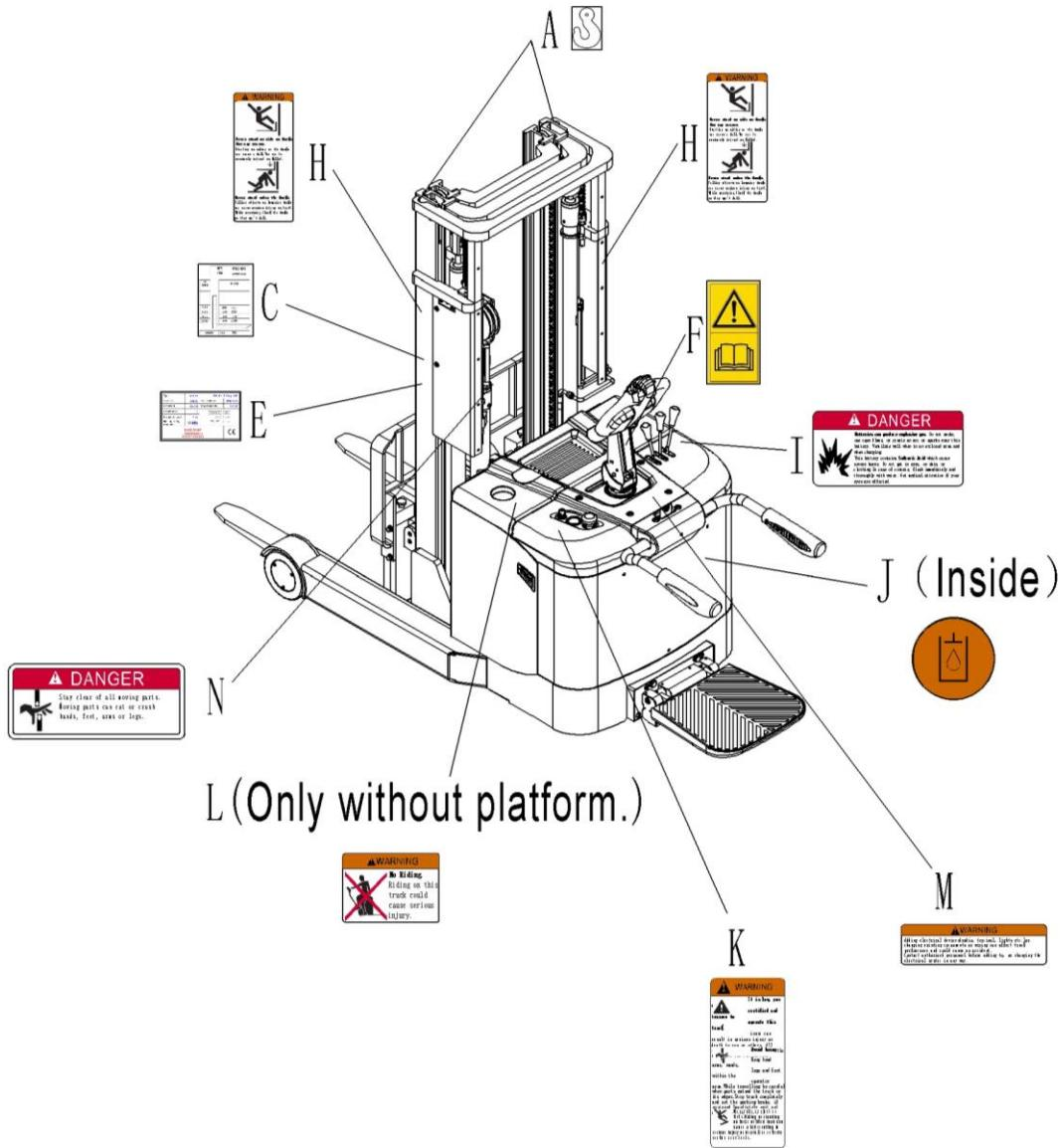
Fig. 18: Warning labels and safety devices (only USA)
