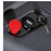
Key Switch, Battery Discharge Indicator, Emergency Switch
