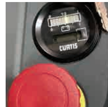
Bat. Discharge/Emergency Switch
