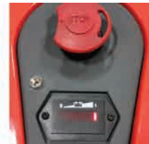
Emergency Stop/Battery Indicator
