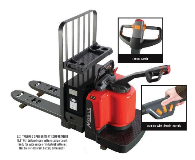
Able to lift and transport loads of up to 6,000 lbs, the HESPT60N self-propelled pallet truck is designed for heavy duty lifting and transporting applications. These units feature full electric lifting and self-propelled movement with an operator platform, enabling safe and more efficient load handling, particularly in long-distance warehouse applications.
