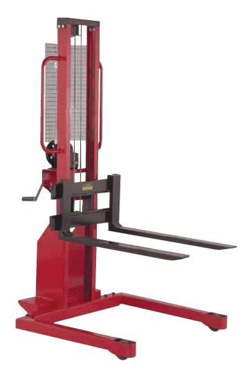
The Mobile MW750 is a compact unit ideal for loading/unloading trucks where docks do not exist. The adjustable straddle legs enable the unit to handle pallets of any size without sacrificing ergonomics. Unit includes: heavy-duty cable to ensure load/lifting safety; an easy-to-turn hand winch with an automatic braking system; a safety cage that protects the operator but still
