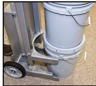
Lifting yoke holds pails in place
